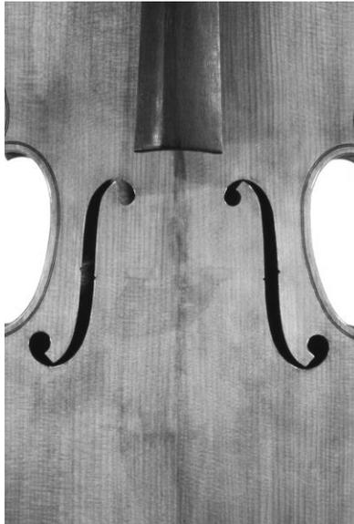
*Fig. 1 Fading of violin varnish that was exposed to 5 foot-candles illuminance for one year. The light source was a single 60-watt, 2800°K quartz-HALOGEN lamp directed from a ceiling fixture through a 1/4-inch-thick PLEXIGLAS® vitrine. Note the distinct “shadows” of bridge, tailpiece, fingerboard, and strings.*
