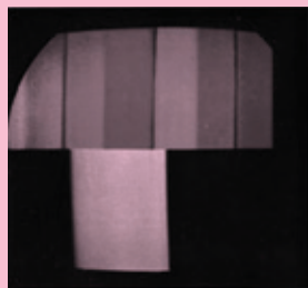
Fig. 12. Photograph of color-bar pattern on color receiver viewed through oscillating screen and zoom
