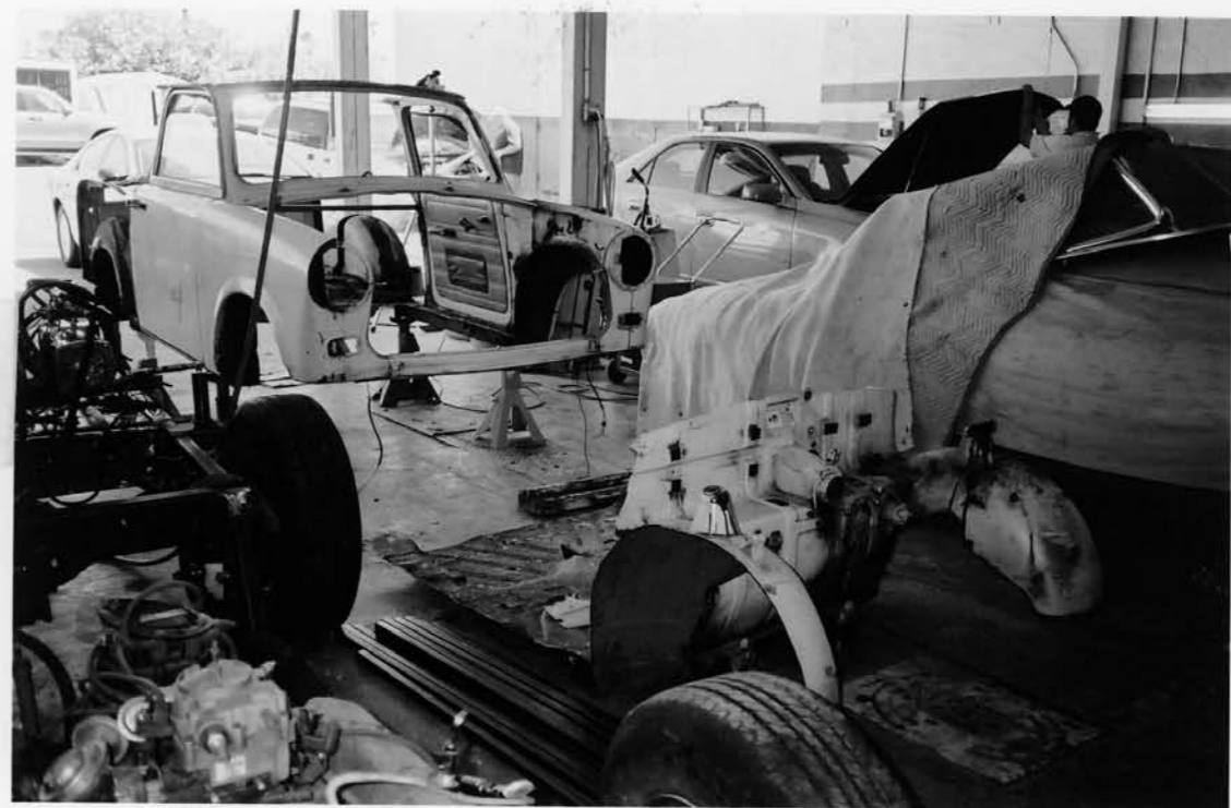
CUTTING OUT FIREWALL & FLOOR TO MAKE ROOM FOR ENGINE & TRANSMISSION
