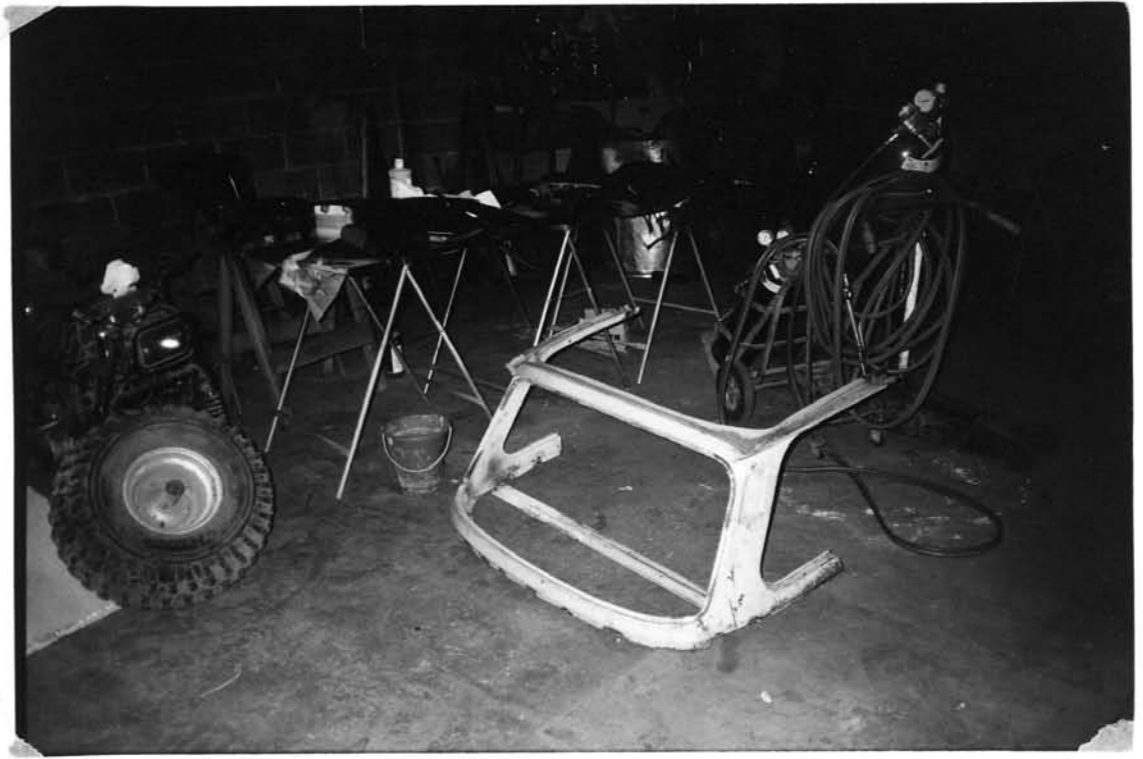
CUT BACK HALF OF PASSENGER CAB. THIS PART WILL SLIDE FORWARD TO MAKE THE EL CAMINO CAB ↘
