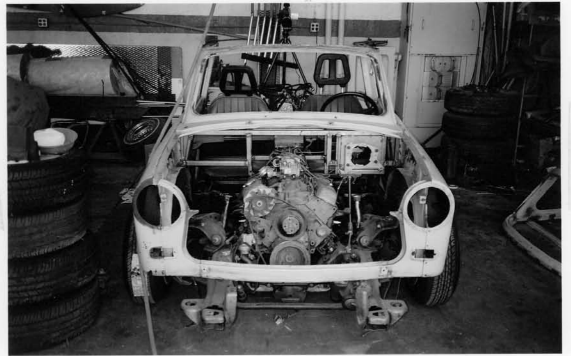
FIREWALL FRAMEWORK & BRAKE BOOSTER BRACKET
