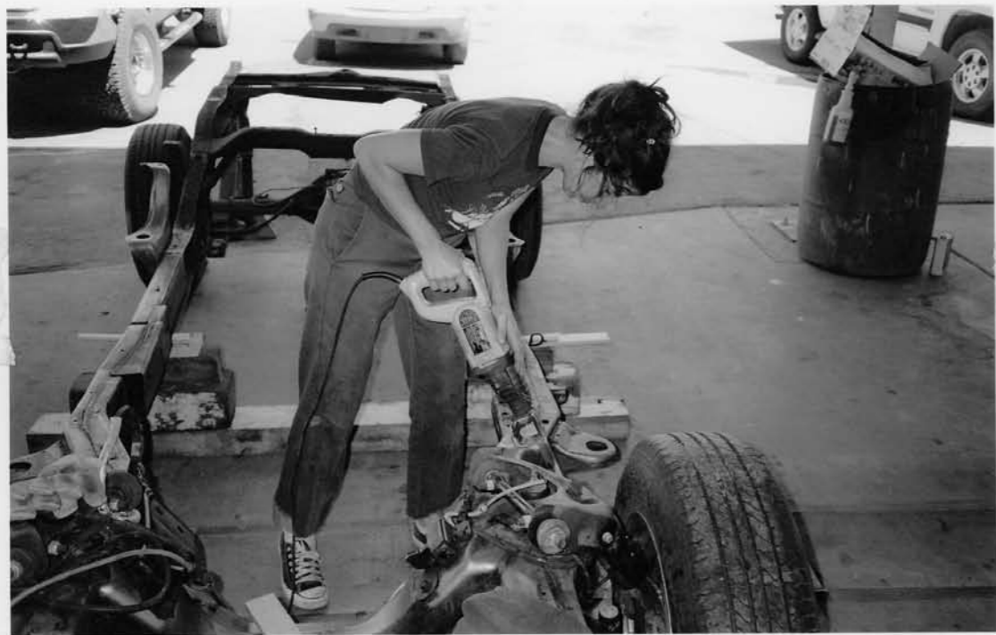
CUTTING FRONT END OFF S-10 CHASSIS TO BE ABLE TO MOUNT A SMALL BLOCK
