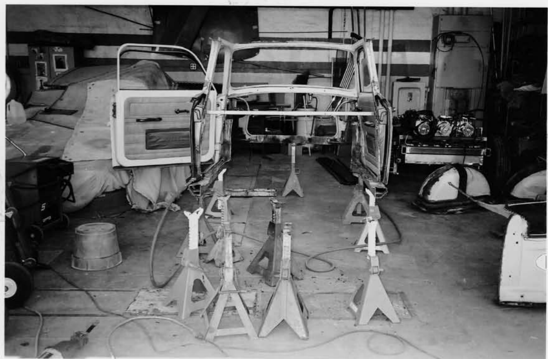
CUT BODY IN HALF TO MAKE EXTENDABLE
