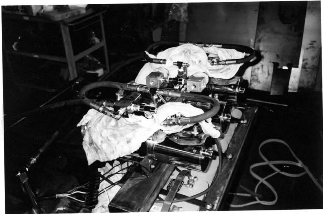
2 OUTER PUMPS FOR SUSPENSION HYDROS. MIDDLE PUMP FOR CHASSIS HYDROS. 6 BATTERIES. 4 FOR SUSPENSION, 2 FOR CHASSIS.
