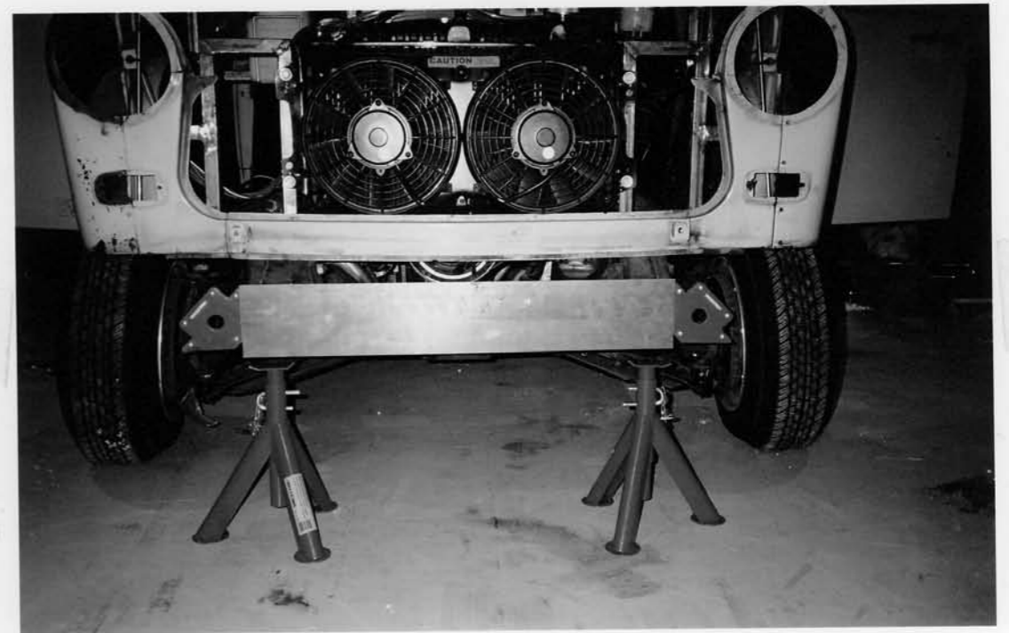
METAL PLATE FOR BUMPER ATTACHMENT
