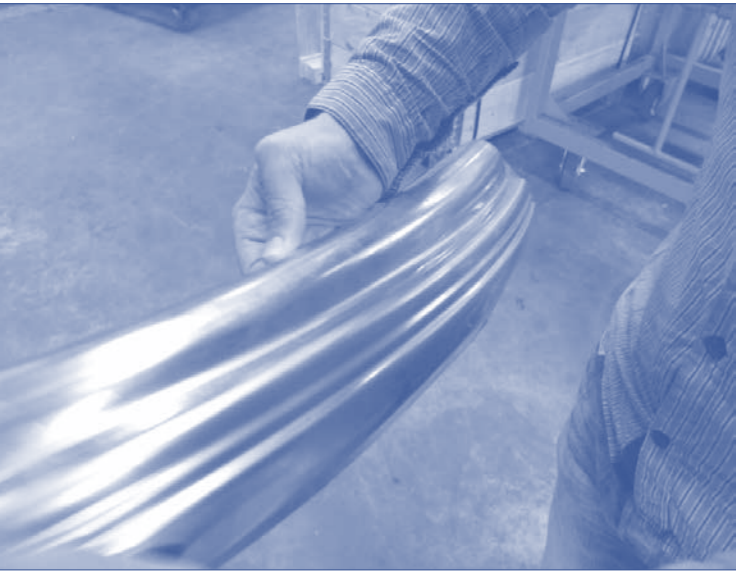
ABOVE : 3D LASER CUT STAINLESS STEEL PANEL
