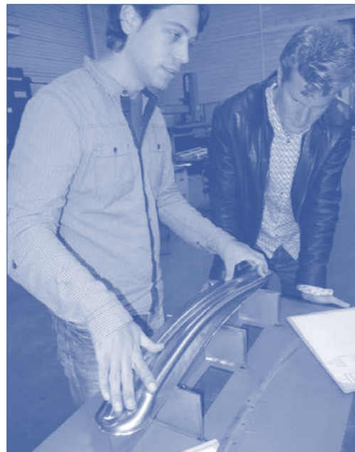
BELOW : PART FITTING IN LASER CUTTING MOULD
