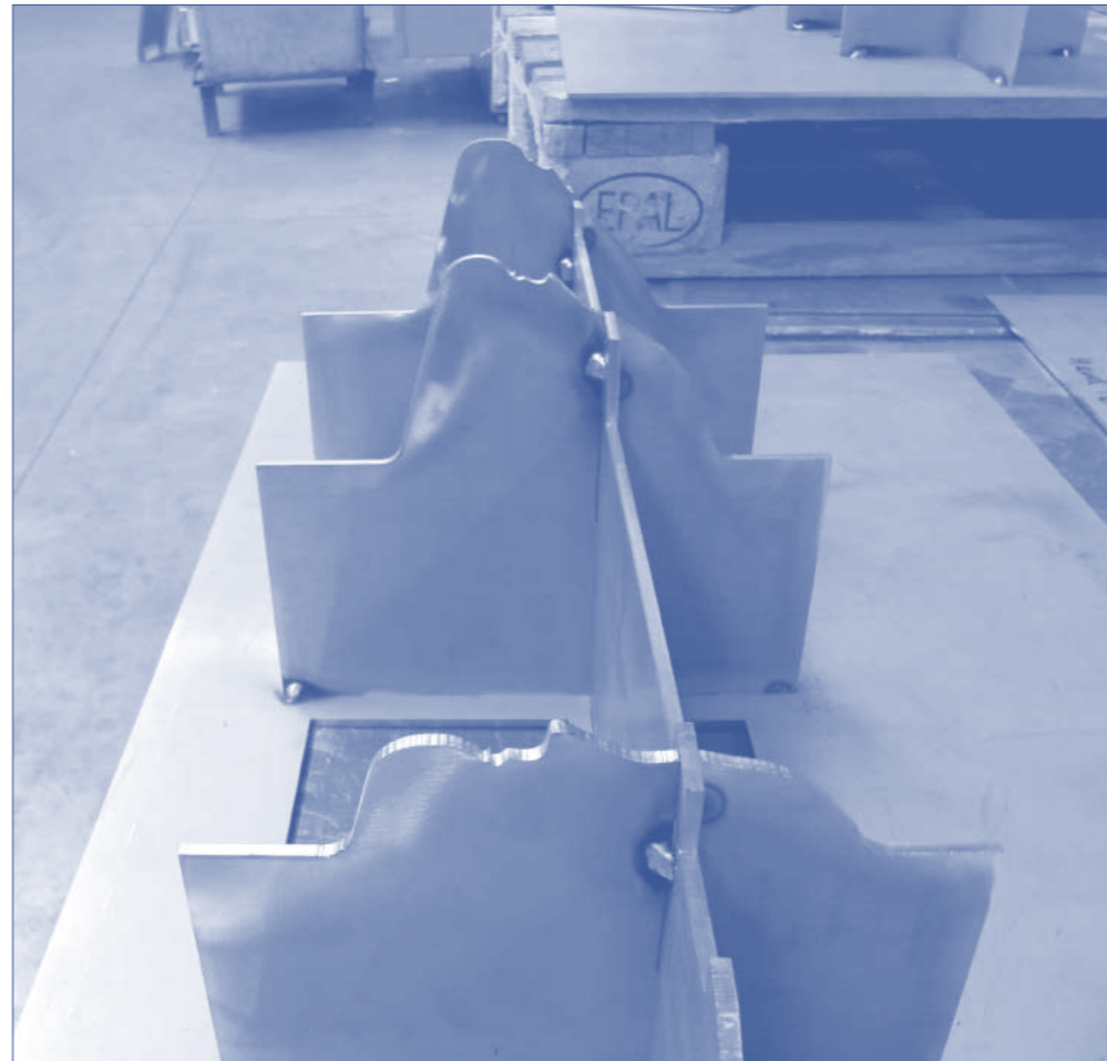
BELOW : EVERY SECTION HAS ITS OWN LASER CUTTING MOULD
